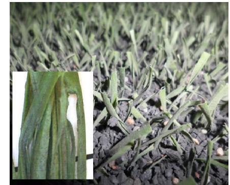
Photo: Drop fiber after 110.000 cycles on 15m lisport
