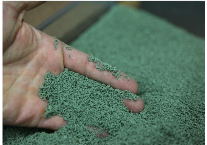
Photo 24: EPDM infill (source: Smart Connection Consultancy)
