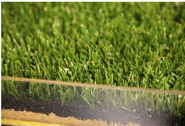
Photo 22: Example of a mixed profile of sand and rubber infill
