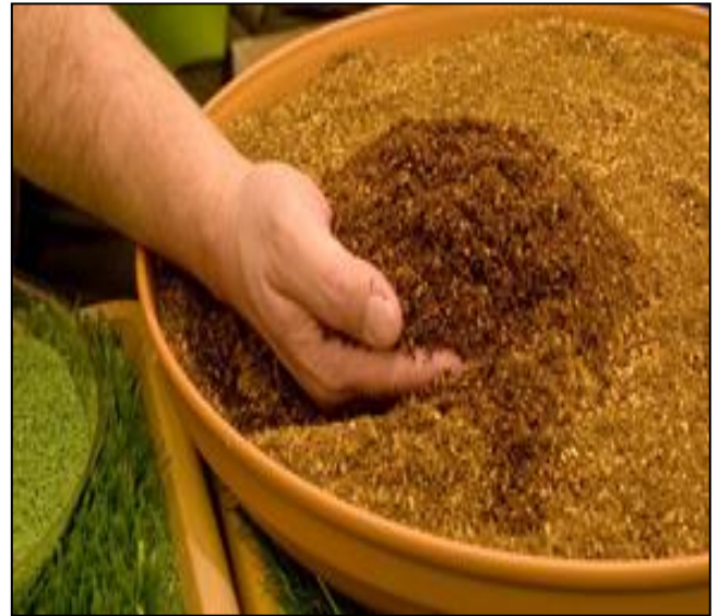
Photo 25: Organic Infill (source: Limonta)
