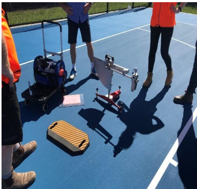
Photo 34: Testing apparatus for slip resistance
