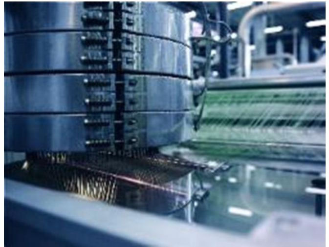
Photo 19: Extrusion Process producing mono-filament yarn
