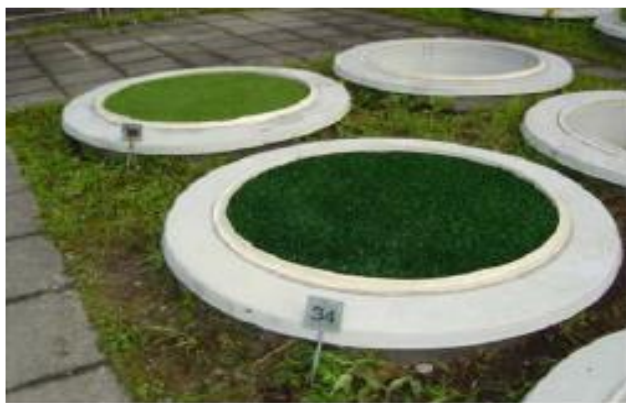
Photo 13: Swiss Study collecting rainwater through various synthetic sports surface systems
