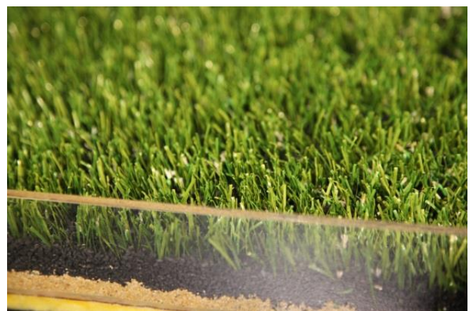
Photo 17: Example of a mixed profile of sand and rubber infill
