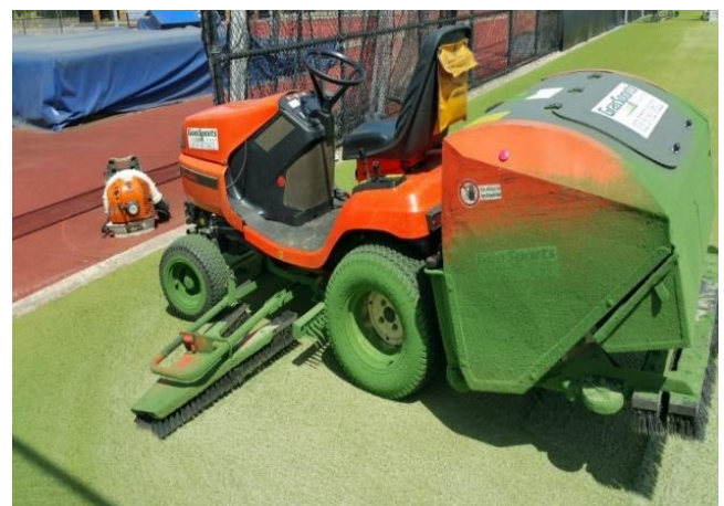
Photo 29: The yarn has been exposed to UV and the tips are breaking down and covering the maintenance machine
