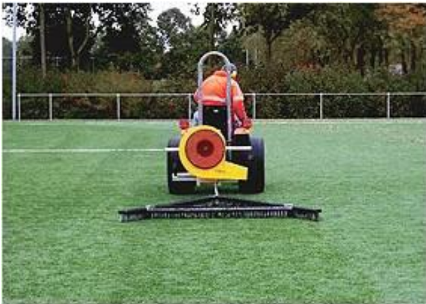
Photo 19: Least impact on Ball Roll was found on the Triangular Brush
