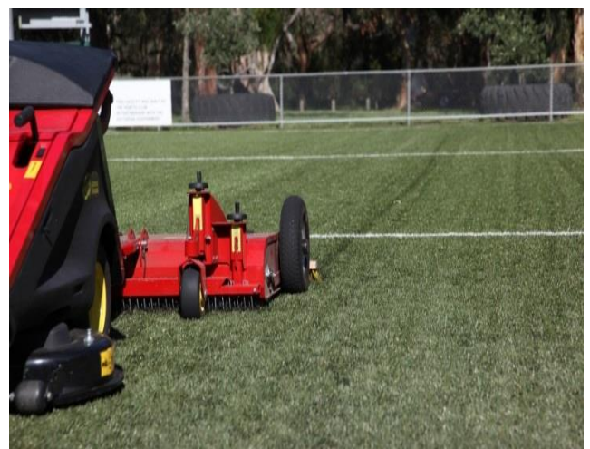
Photo 23: Tines being used to decompact infill and redistribute infill
