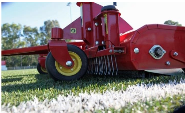
Photo 27: Modern machine providing height options for the Tines to be used into the turf by an experienced operator
