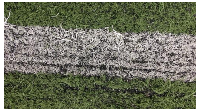
Photo 17: UV degradation of white lines in Melbourne Football field
