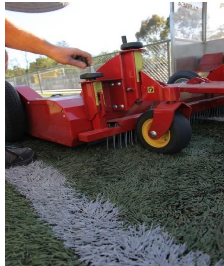
Photo 20: Setting the tines length to decompact a flat grass surface
