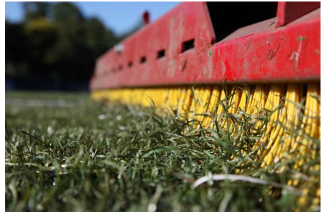
Photo 26: Brushes towed behind small tractor machine is better than a drag mat
