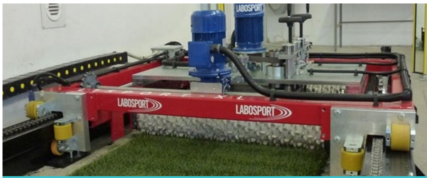
LisportXL durability testing machine (Labosport)
